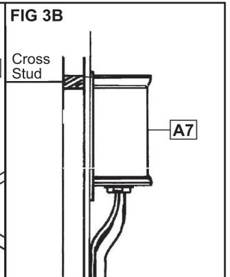
**5** Align hanger brackets (B) on the wood tank to the inside notch of the molding bracket (D) and hang the wood tank (A7). (Fig 3B)
