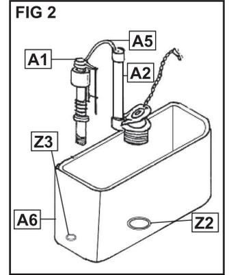
**3** Make sure and check that the refill tube (A5) is inserted on top of the overflow pipe. (Fig 2)
